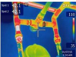
Thermal Image of water and space heating piping in a resident unit (red = heat escaping)
