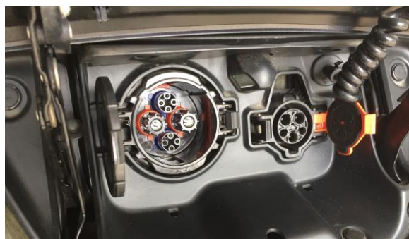
CHAdeMO DC receptacle (left) and J1772 AC standard receptacle (right). Source used with permission from: https://images.nrel.gov
