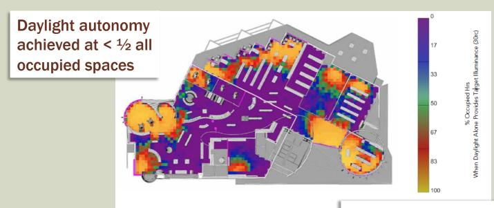
Daylight Autonomy - Daylight Levels of 30fc at floor
