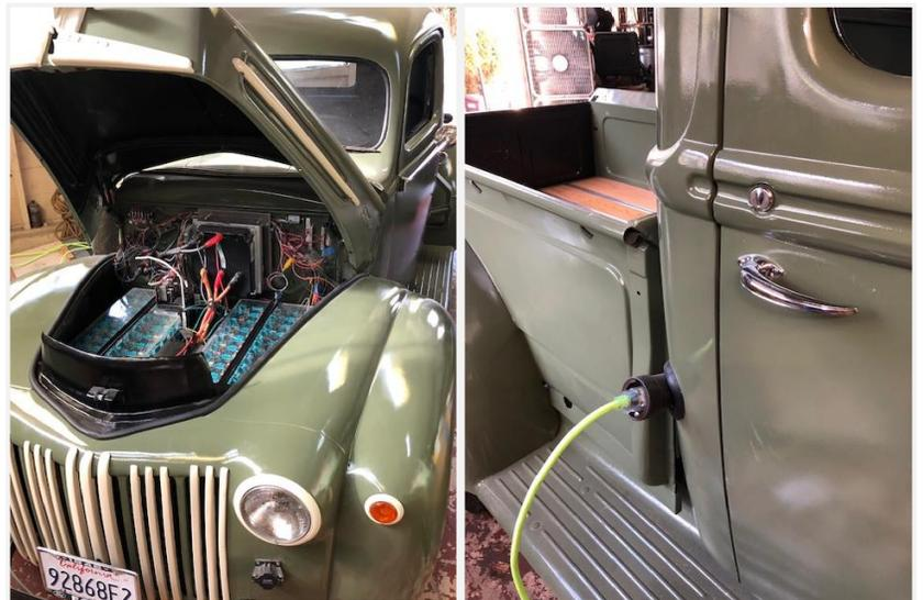
Figure 38: Electrified 1946 Fork Pickup truck.<sup>121</sup>
